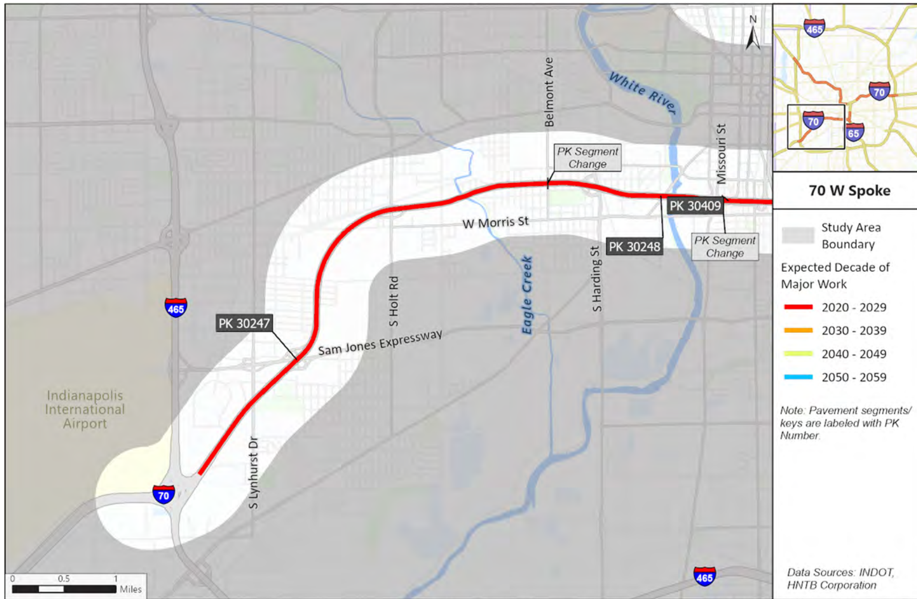
Figure 13: 70 W Spoke Expected Major Pavement Work by Decade
